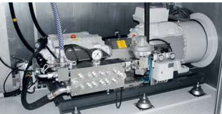
Test pump unit DP724 E for cyclic pressure testing in container design.
