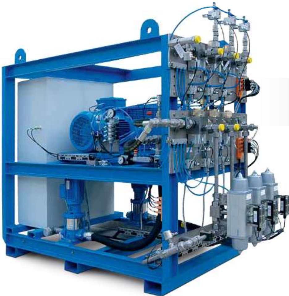
Fully automatic test pump unit DP3-10 E with filling and test function for several test points with different testing pressures and volumes
