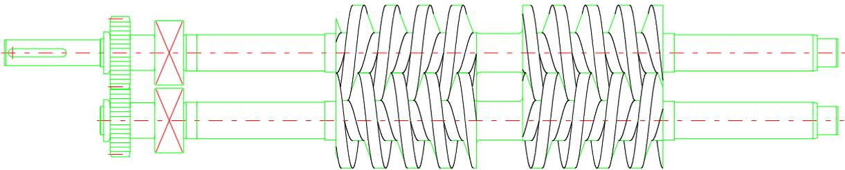
Fig. 1.1 Screws with timing gears
